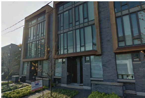
Walls incorporated into the design to screen utility meters.
